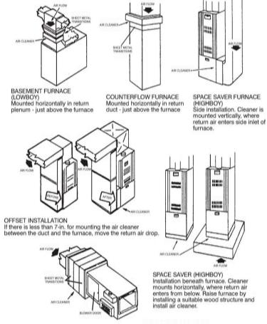
HORIZONTAL FURNACE Mounted vertically in return duct as close to the furnace as possible
