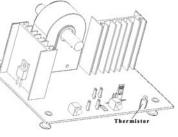
which when electrically powered heats up to approximately 130° F. The AFS stabilizes at this temperature and while the HVAC system blower is in operation, air flows through the ductwork, creating a vacuum effect that pulls cooler air over the hot surface of the thermistor. This air movement cools down the thermistor which allows the AFS to register that the HVAC system blower is moving air and the Electronic Air Cleaner must be powered to provide air cleaning.
