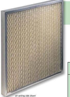
Multi-Pleat HT filters are designed for ovens and air filtration systems with continuous operational temperatures up to 500°F (260°C). This product is widely used in applications such as paint spray booths, baking systems, drying ovens, and in any system where elevated operating temperatures require a more specialized type of air filtration.
