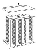
Double Header Model DuraMAX 4v is offered in two header designs. Standard single header (above), and double header model (left) for housings requiring double header configuration for proper installation.
