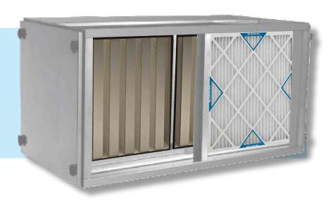
The **BioMAX HEPA Lock Housing** is constructed of 16 gauge galvanized steel. It is also available in aluminized, stainless steel and epoxy coating, which provides superior corrosion and heat resistance.
